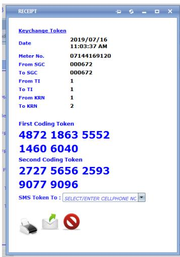
Punch in the first 20-digit token “coding token” (meter will flash (scroll) in left hand corner of the screen above the smiling face)
