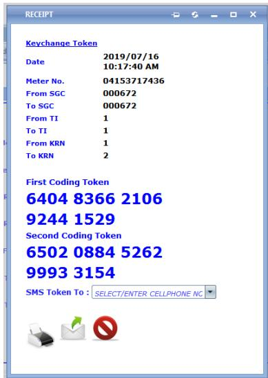
1. Punch in first set of 20 digits “coding token” – the meter will flash (5 sec) , continue to next step
