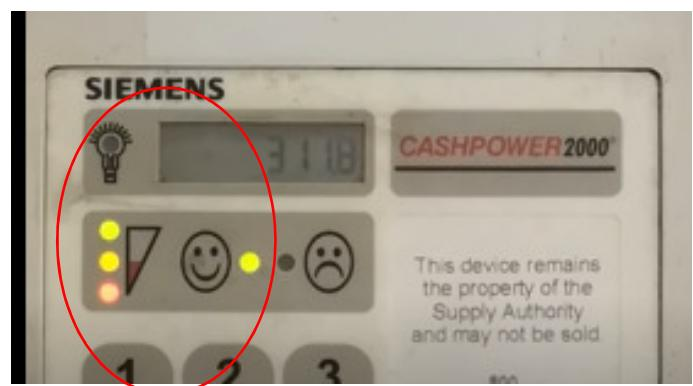
Punch in the Second 20-digit token “coding token” (meter will flash (scroll) in left hand corner of the screen above the smiling face) (meter will display 2.2 in right hand corner)
