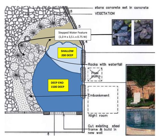
b) complete with natural water rock feature rear wall, with a small drinking pond flowing into waterfall over feature wall. Length 3.0-3.5m x 0.35-1.0m high x 0.5-0.75m wide. Water fountain to cascade from drinking pool to water pool. Rock feature to be wide enough to create platform for Jaguar to lie down.
