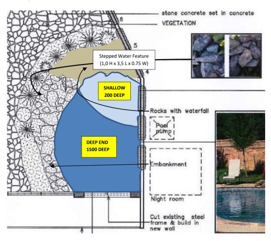
b) complete with natural water rock feature rear wall, with a small drinking pond flowing into waterfall over feature wall. Length 3.0-3.5m x 0.35-1.0m high x 0.5-0.75m wide. Water fountain to cascade from drinking pool to water pool. Rock feature to be wide enough to create platform for Jaguar to lie down.
