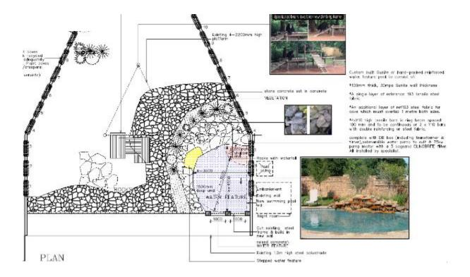
a) New Gunite swimming pool approximately 3500 x 4500mm in size. The swimming pool has two levels, a shallow level 3500mm x 1000mm x 200mm deep; then a deep end of 1500mm. The pool will be raised above ground level about 1000mm high to accommodate viewing window as per architectural design.
