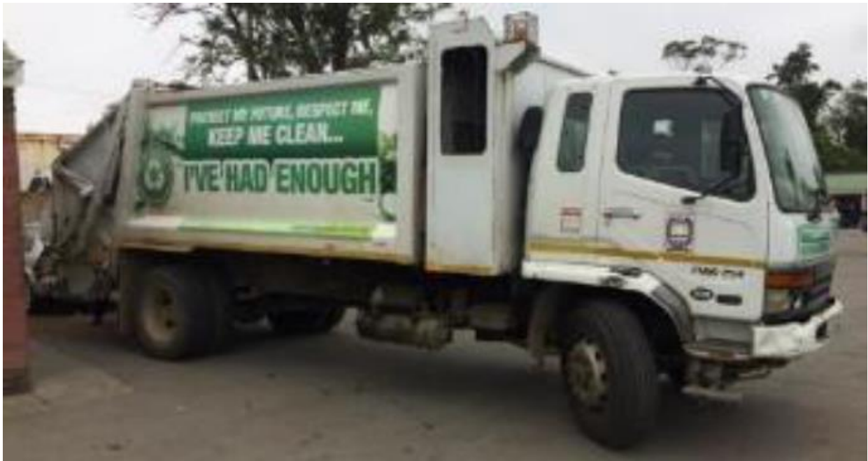
Figure 22: Rear End Loader waste compactor in KWT
