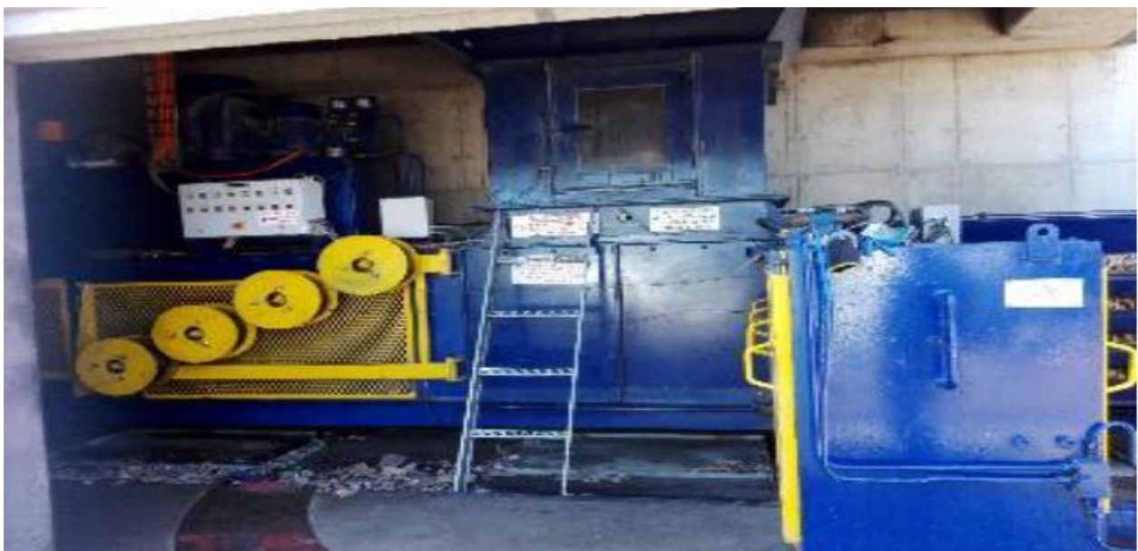
Figure 17: Collect-All's Granulator to process plastics into chips for sale to market
